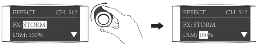
Rotate "Right knob" to select from DIM, CCT and INTVL.
