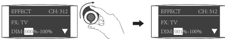
Rotate "Left knob" to adjust the value of DIM, CCT and SPD.
