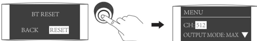
Press "Right knob" to confirm reset and it will return to the menu after bluetooth reset.
