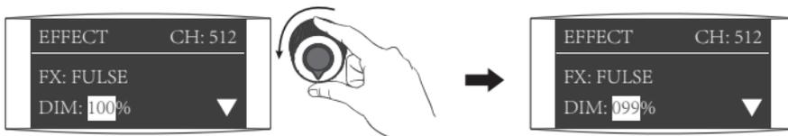
Rotate "Left knob" to adjust the value of DIM, CCT and PULSES/MIN.
