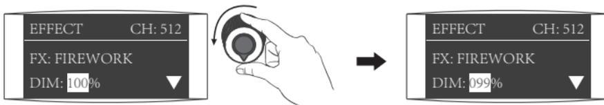
Rotate "Left knob" to select from DIM, CCT, SPD and DECAY.
