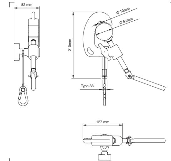
BABY PIPE CLAMP WITH 16MM STUD **C210**
