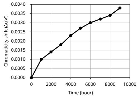
1. Data from IESNA LM-80-2008, report number R2DG150122050-10-9000. The data is based on individual LED of 100% rated current, the LED on the strip works at typical 50% rated current.
