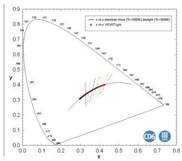
Shown on the diagram are the VELVET lamp head chromaticity coordinates (x, y CIE-1931) feed and digitally controlled by its Control Unit and they are compared with the reference illuminants. These reference illuminants are the Planckian locus radiator set below 5000K and the CIE daylight reference is set over 5000K. The Planckian locus radiator references the chromaticity for several tungsten lamps colour temperatures while the daylight locus typify daylight type D illuminants.
