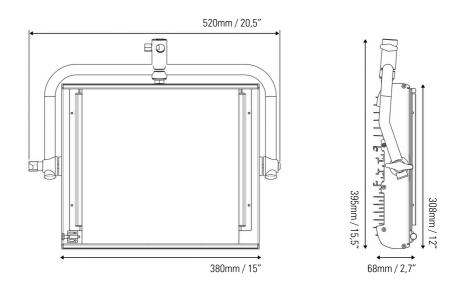
**VELVET Power 2** Weight: 7 kgs / 15,5 lbs. Power draw 190 W /1,7 Amps at 14,4 VDC. FLOOD/SPOT IP51 protection
