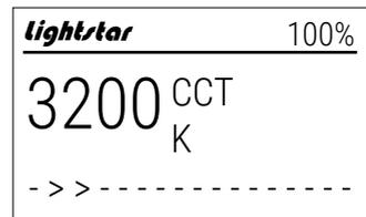
Figure 3 - Temperature Adjustment
